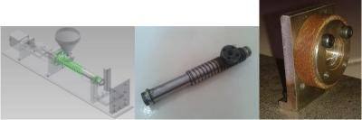
Figure 13 CAD Drawing and Manufactured Products of Injector Barrel and Flange
