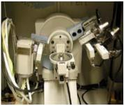
Fig.3.10(b) FXPERT XRD with X'celerator Detector for thin film
