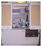
Fig.3.10(a)X'Pert pro Multipurpose Diffractometer (MPD)
